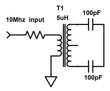
An IF can (T1) used in this configuration needs the core slug of T1 to set the value of the inductor at c. 5uH, for resonance at 10MHz.
