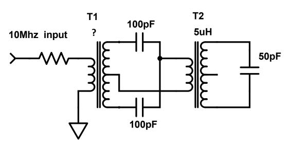
The primary of a second identical IF can (T2) is added between the centre tap of T1 secondary, and the junction of the 2  $\times$  100pF capacitors....
